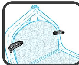
3 Hand tighten the two front plate brackets. Be aware: Do not tighten until sidepanels are attached!
