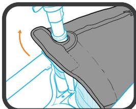
4 Pull the velcro ends together behind the steerer tube.
