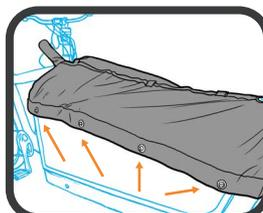
2 ...tension fabric using the attachment points on the side panels.
