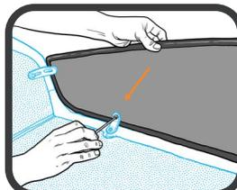
1 Attach both side panels using the grub screws and ensuring they are aligned to the frame.
