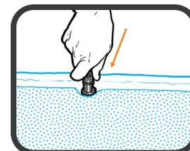
2 Insert the four brackets with rubber O-rings into the frame holes.
