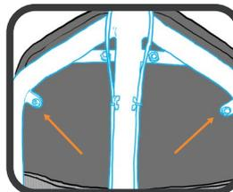
3 ... using the four attachment points. Be aware: Only hand tighten the thread locked nuts!
